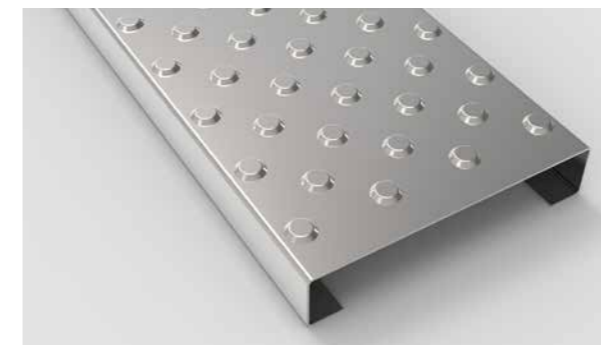
Type AP 2 - 50 closed (NOP) Type AP 3 - 50 closed (NOP) Embossed \varnothing 16 mm dome 4 mm high on a 50 mm staggered pattern. Also available with drainage perforation \varnothing 8 mm if required.
