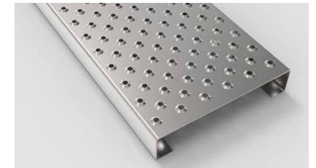
Type AP 2 - 30 without drainage (ZAW) Anti-slip perforation Ø 8 mm punched up 3 mm high on a 30mm c.t.c staggered pitch. No drainage perforations
