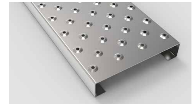
Type AP 2 - 50 without drainage (ZAA) Type AP 3 - 50 without drainage (ZAA) Embossed dome with \varnothing 8 mm perforation punched up 3 mm high. No drainage holes.
