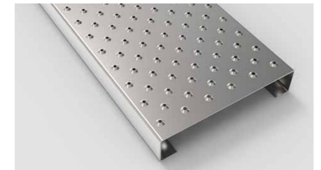
Type AP 2 - 30 safety without drainage (VZA) Anti-slip perforation Ø 5 mm punched up 3 mm high on a 30mm c.t.c staggered pitch. No drainage perforations
